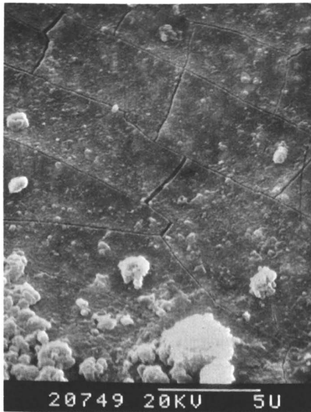
Figure 6. Micrograph of B in Table I. acceleration test; 700 hrs., magnification bar; 5\mu .
